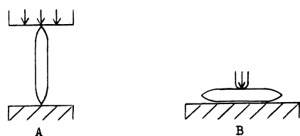
Fig. 2. Crushing direction of an ampoule containing a sample.
